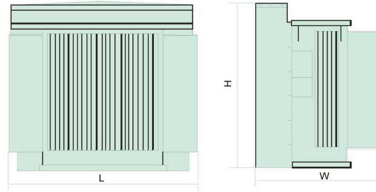
额定电压 Rated voltage: 6, 6.3, 10, 10.5/0.4kV
